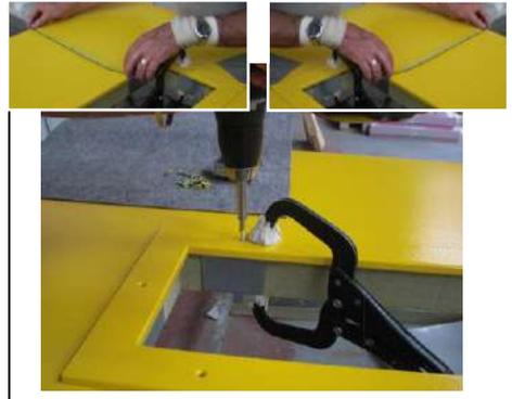
Secure the ring to the blade using a pressure clamp and screw it into the holes provided with the screws supplied.
