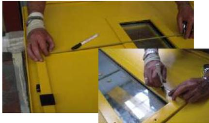
9.- Cut and place the ceramic blanket. Drill in correspondence of the marks previously made.
