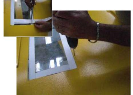
10.- Place the ring and screw it into the previously drilled points, **taking care not to tighten it too much so as not to damage the glass.**
