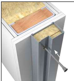
2. In order to fix the frame to the wall, we insert the corresponding screws, passing through the hole provided in the frame and the hole provided in the fixing plate until it is anchored in the wall.
