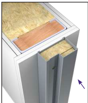
1. Level the frame on the wall.
