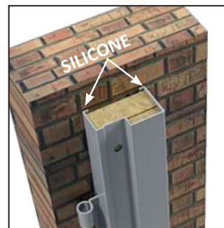
3. Once the screws are anchored in the wall, both edges of the frame are sealed with silicone. If there is a gap between the frame and the wall, it must first be filled with rock wool and only then sealed with silicone.
